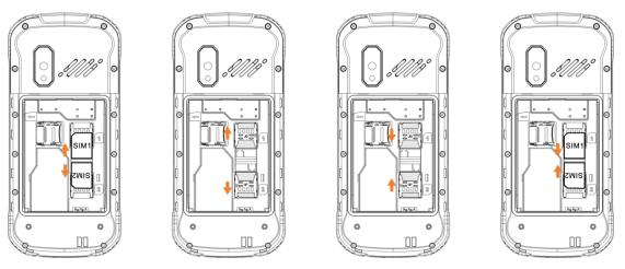
Place the SIM card with the chip facing downwards and slide it into its housing. Make sure that it is correctly inserted. To remove the card, press it and slide it out
