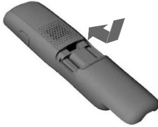
2. Align the cover flat against the battery compartment, and then slide it upwards until it clicks into place.
