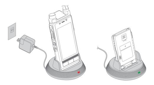
To determine the charging status, check the LED indicator on the charger according to the following table:
