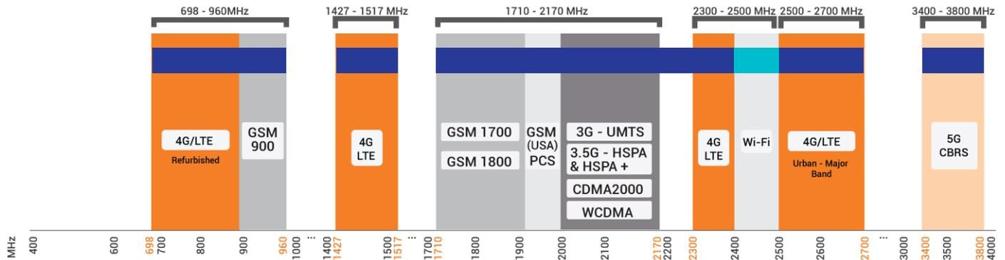
Indicates the 5G/LTE bands on which LPDA-92 works      Indicates the WI-FI bands on which LPDA-92 works
